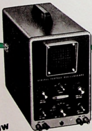
HEATHKIT OSCILLOSCOOP 10-21 E (110-220 V.) "GENERAL PURPOSE"
